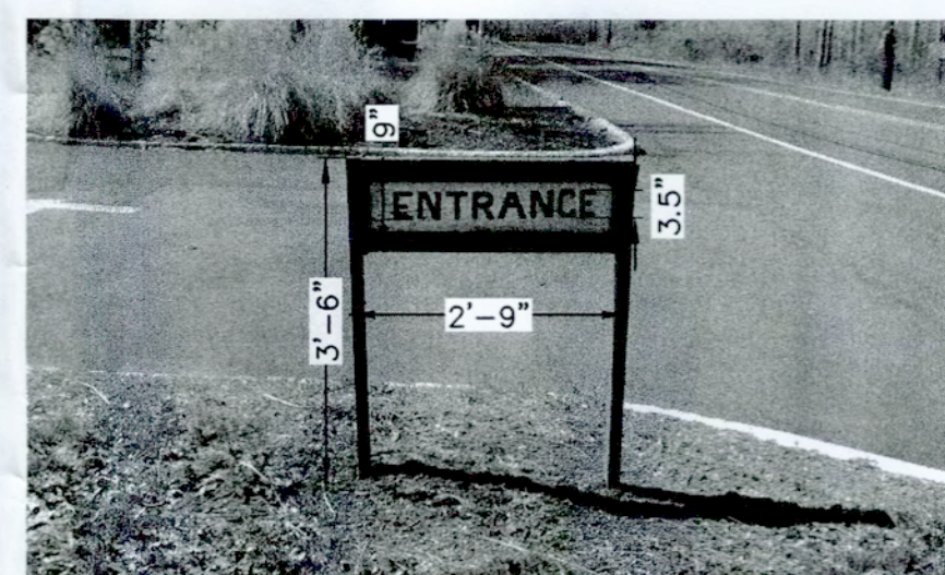
"ENTRANCE" & "DELIVERIES" SIGN DETAILS N.T.S.
